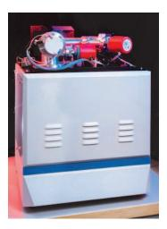
The mass spectrometer can be 'tuned' to different masses of gas molecules. In practice where a mass spectrometer is fitted with a fixed radius flight tube and a permanent magnet, this is accomplished by varying the acceleration voltage of the ion source. In systems fitted with electromagnets the magnetic field intensity can be varied.
