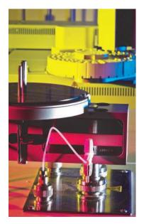
This is probably the most common elemental analyser configuration which determines total carbon, hydrogen and nitrogen simultaneously. It is well suited to the analysis of most organics and inorganics from 0.01% to high percentage levels. The CHN method is limited to the analysis of relatively small sample weights because the resolution of the nitrogen and carbon peaks can be compromised.
