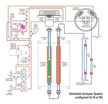
Unlike CHN or CHNS analysis modes the NC method has almost unlimited resolution of the nitrogen and carbon peaks which allows the analysis of much larger samples. See the Weight Requirement Guide for Sample Submissions Table earlier in this section. Where the NC values are likely to be very low (in soils for example) it is possible to use higher sample weights and/or increase the gain of the instrument to achieve a better signal to noise ratio.
