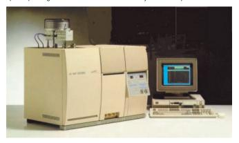
The CHN method is limited to the analysis of relatively small sample weights because the resolution of the nitrogen and carbon peaks can be compromised. See the Weight Requirement Guide for Sample Submissions Table earlier in this section. Where the CHN values are likely to be very low it is possible to use higher sample weights and/or increase the gain of the instrument to achieve a better signal to noise ratio.
