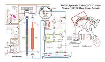
An **elemental analyser** is a sample preparation unit used to convert solid or liquid samples into gases suitable for analysis by mass spectroscopy. Nitrogen, carbon and sulphur are converted into  $N_2$ ,  $CO_2$  or  $SO_2$  by combustion, oxygen to CO by high temperature pyrolysis and hydrogen to  $H_2$  by high temperature reduction.
