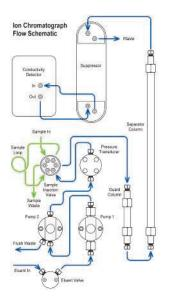
A two stage pump constantly pumps the eluent (usually a 9mM aqueous solution of sodium carbonate) at high pressure (~2000 psi) through the ion chromatography system.
